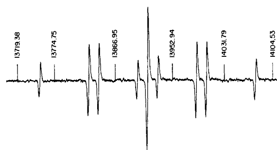
Figure 2. ESR spectrum of (\text{C}_2\text{H}_5)_3\text{SiCH}_2\dot{\text{C}}\text{H}_2 obtained by addition of (\text{C}_2\text{H}_5)_3\text{Si} to ethylene at -148^\circ .
